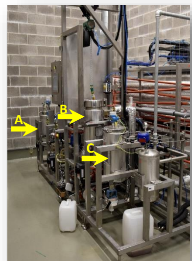
Figure 2: extraction pilot for subcritical water use. A: water tank; B: Reactor; C: extract collector
